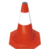
Model:RB-500A Height:500mm Weight:1.5kg Base Size:350X350mm Reflective band size:140mm
